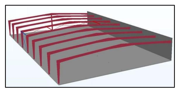
Shear walls are structural members, typically composed of pre-cast or tilt-up concrete wall panels, which are used to resist the building longitudinal forces.
