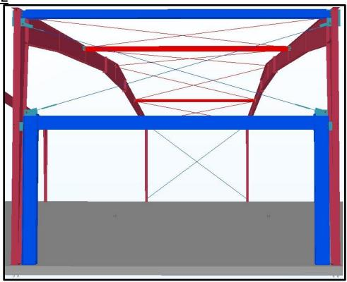
Portal Frames are rigid frames that span in the longitudinal direction between primary rigid frames. Portal Frames are an alternative longitudinal bracing solution that replaces standard X-Bracing in one or both sidewalls with Portal Frames. Portal Frames are options where a desired clear height or clear width must be met in a sidewall bay. Due to their inherent flexibility and greater mass, Portal Frames are a more expensive longitudinal Bracing option than full height X-Bracing.
