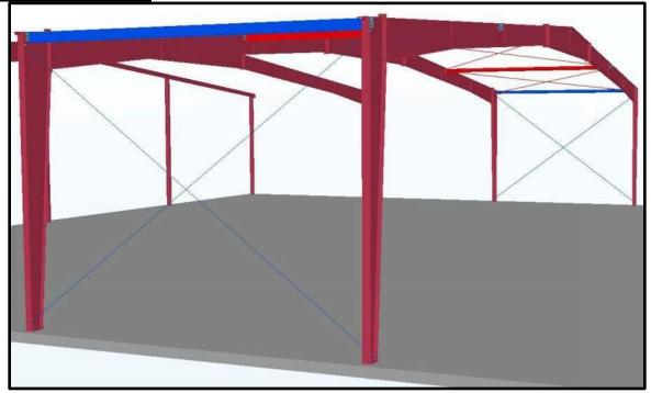
Full height X-Bracing is the standard Valley Steel Building System solution to longitudinal strength and stability and is the lowest cost option. The below guidelines are intended to provide guidance when utilizing full height X-Bracing.
