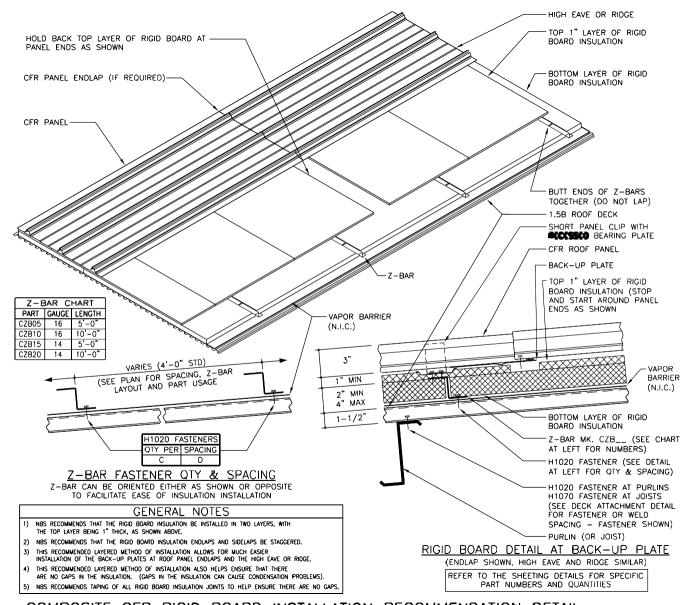
COMPOSITE CFR RIGID BOARD INSTALLATION RECOMMENDATION DETAIL Z-BARS AND 1.5B DECK
