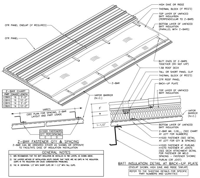
COMPOSITE CFR BATT INSULATION INSTALLATION RECOMMENDATION DETAIL Z-BARS AND 1.5B DECK
