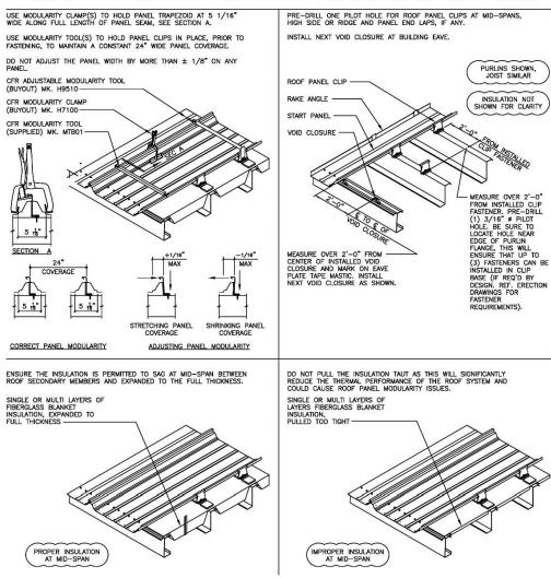
GUIDANCE TO INSTALLING SINGLE OR MULTI LAYERS OF INSULATION WITH "CFR" ROOF
