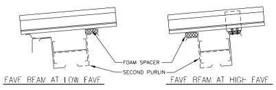
IF THIS PROJECT HAS AN EAVE BEAM WITH (2) PURLINS, AS SHOWN,  $\underline{\text{DO}}$   $\underline{\text{NOT}}$  ATTACH ROOF CLIPS TO THE "SECOND" PURLIN. HOWEVER, EPS FOAM SPACER IS PROVIDED FOR INSTALLATION AT THE SECOND PURLIN.
